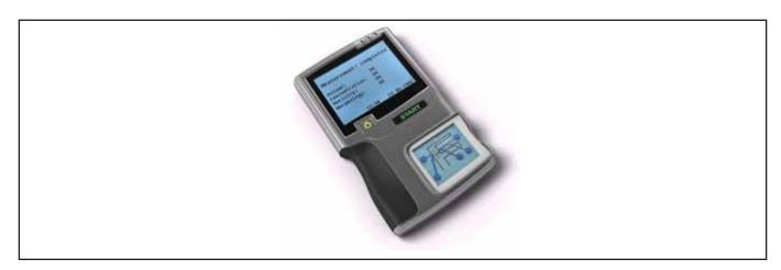
Figure 1 An artistic impression of the fertility chip. It consists of a handheld system, microfluidic chip and software.
